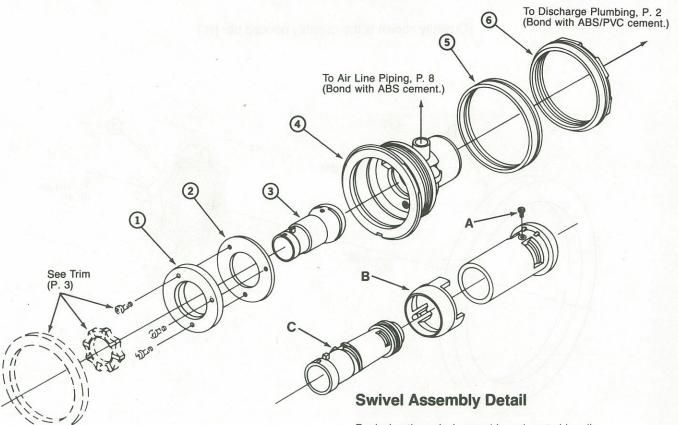
Replacing the swivel assembly and venturi handle:
