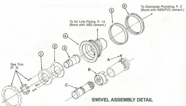
Replacing the swivel assembly and venturi handle:
