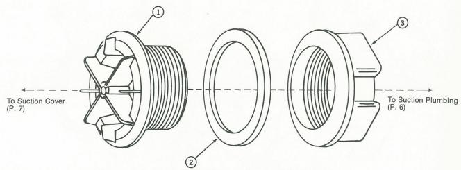
Do not use #1836000 Back-up Ring from AMH Jet. Use of non-interchangeable parts may cause leaks or malfunction.
