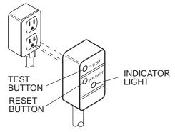
1. The spa is supplied with a 15 foot line cord which terminates with an integral GFCI plug. Locate the spa near enough to a weather protected outlet, but no closer than 10 feet. DO NOT USE AN EXTENSION CORD! Using an extension cord is hazardous and will decrease the amount of power to the unit, causing slow heating, poor whirlpool performance, or system malfunction.
